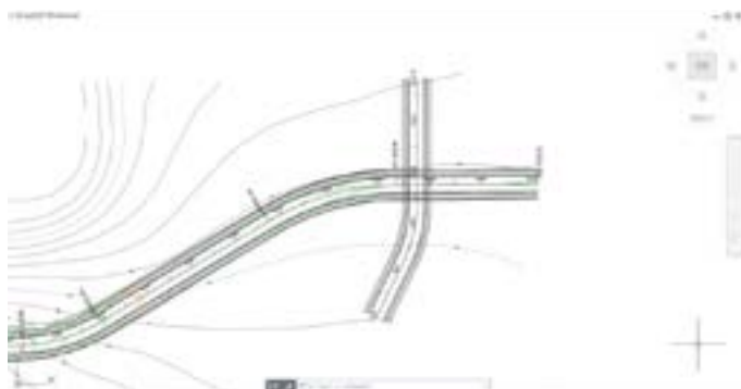
Laying out an intersection in AutoCAD.
