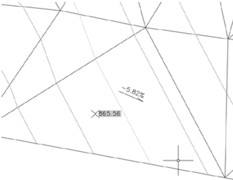
Spot elevation and slope labels in AutoCAD
